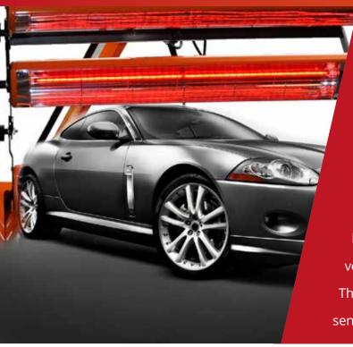
Victory's Heatlight range of large paint dryers utilises 1 & 1.5kW glare control lamps, configured in individual cassettes to yield up to 6kW of drying heat. The lamps emit short wave infrared heat which is ideal for optimising drying of water-based paints. These flexible systems allow each cassette to be adjusted and locked into position around the contours of the vehicle body, ensuring maximum area coverage. There are also options for temperature/distance sensors for ultimate controllability.
