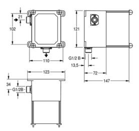
Basic installation kit for FLUSH-C manually operated and FLUSH-S non-touch, opto-electronically controlled urinal flush valve DN 15 for installation in walls. With wall mounting box and function block with integrated lockable water quantity regulator as well as remove plug for flushing and pressure testing.
