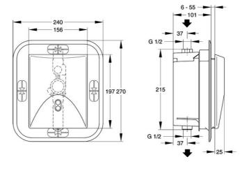
PROTRONIC - A3000 open non-touch, opto-electronically controlled urinal flush valve DN 15 for installation in the wall, with facility for externally controlling the options such as fitting settings and communication via ECC function controller. Adjustable flushing time down to the second.
