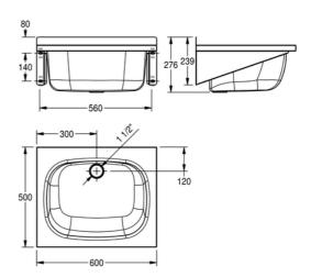
General purpose sink for wall mounting, stainless steel, surface satin finished, material thickness 1 mm, seamless welded bowl with dimensions 500x380x230 mm, rounded edges, 40 mm rear upstand, 1 1/2" plug waste with plastic overflow pipe, drainage back centric, prewelded mounting brackets, incl. stainless steel screws and dowels.
