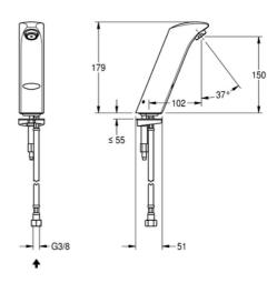
PROTRONIC-S battery-supplied washbasin tap with touch-free operation, DN 15 with aerator and integrated flow control, for connection to pre-mixed warm or cold water supply, polished chromium-plated brass, 6 V battery. WRAS approved.
